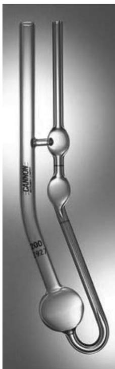
Fig. 3.6. Kinematic viscometer tube from Fisher Scientific.
