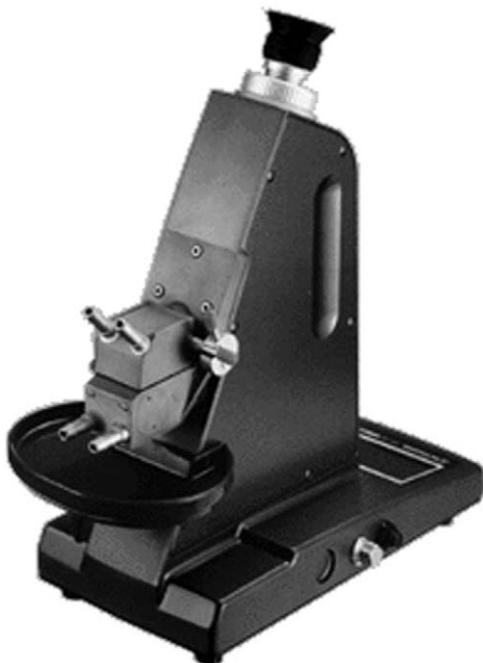
Fig. 3.12. An older Abbe refractometer. Thermostatted water enters and exits through the tubes on the front. The front housing also opens to allow sample to be placed between two analyzer plates.
