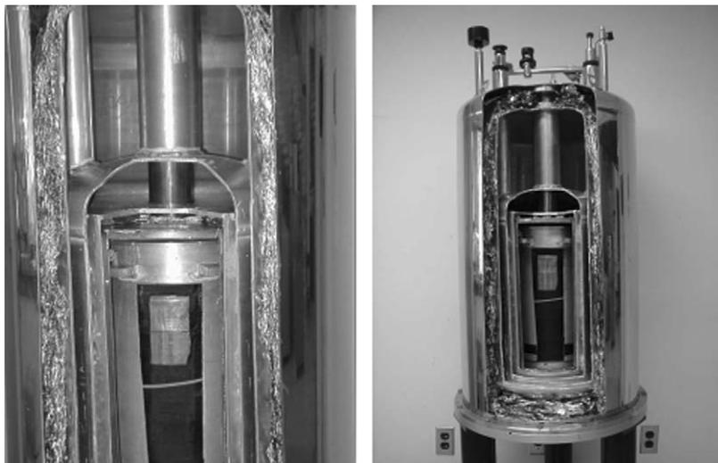
Fig. 10.3. Pictures of a dissected NMR dewar for a superconducting magnet. Pictures taken from [http://www.joel.com./nmr/mag\\_view/magnet\\_destruction.html](http://www.joel.com./nmr/mag_view/magnet_destruction.html), permission not obtained.
