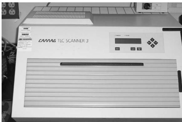
Fig. 13.9. TLC Scanner 3 or densitometer.
