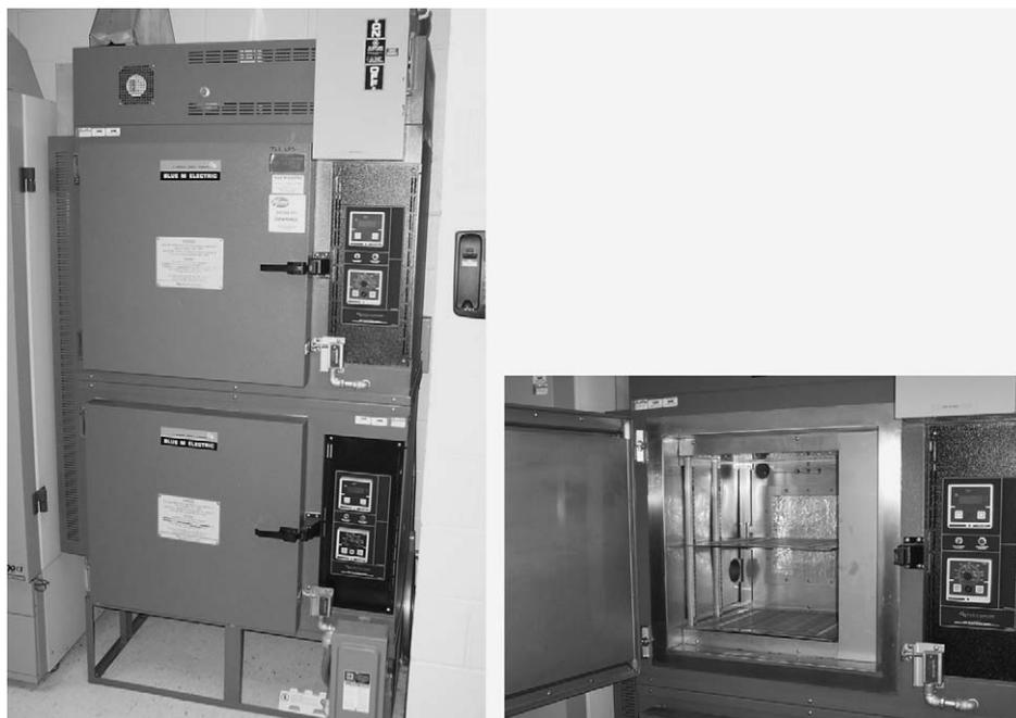
Fig. 13.3. Two views of a typical TLC oven.
