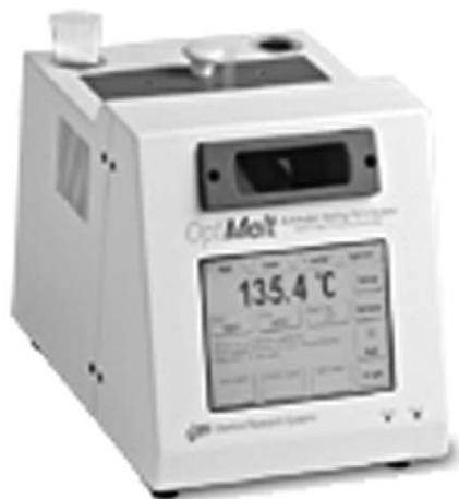
Fig. 3.5. OptiMelt MPA100—Automated Melting Point System. This instrument has automatic and visual determination of melting points. There is PID-controlled temperature ramping and a digital movie is taken of each melt.
