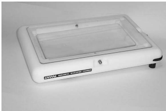
Fig. 13.13. Horizontal developing chamber.
