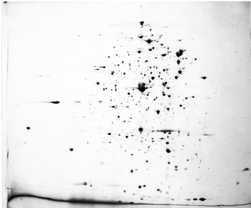
FIGURE 5 Two-dimensional separation of a mixture of denatured peptides from a rat's liver. The separation horizontally is by isoelectric focusing (Section III.D) with the low pH to the left. The vertical separation was made by SDS-PAGE according to size, the largest at the top. (The upper limit of relative mass is \sim 10^5 and the lower limit is \sim 15,000 .)
