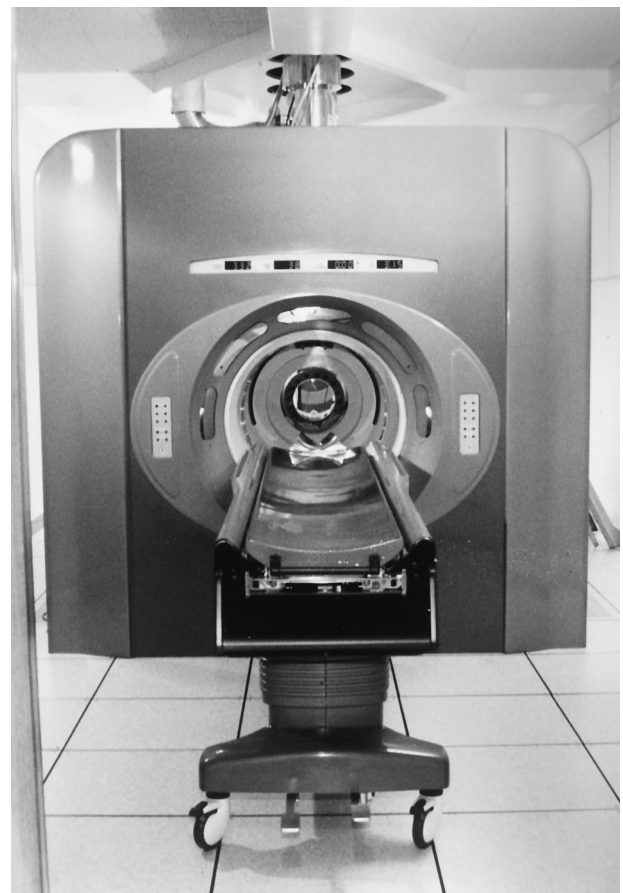
FIGURE 20 Eight-Tesla whole-body magnet. This scanner was installed at Ohio State University in Columbus Ohio in December 1998 for use in MRI research. It is, at present, the highest field whole-body MRI system. (Courtesy of Dr. Pierre-Marie Robitaille.)
