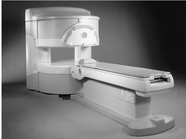
FIGURE 19 High field open magnet. In order to produce field strengths above those achievable with conventional electromagnets, some open scanners, such as this one designed to operate at 0.7 T, utilize superconducting coils to energize the pole faces of the magnet. (Courtesy of Patrick Jarvis, General Electric Medical Systems.)
