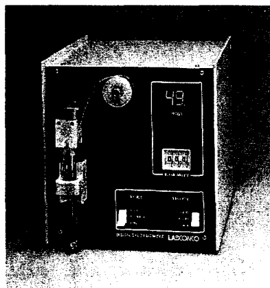
FIGURE 24-11 A commercial digital chloridometer. This coulometric titrator is designed to determine chloride ion in such clinical samples as serum, urine, and sweat. It is used in the diagnosis of cystic fibrosis. The chloridometer is also used in food and environmental laboratories. (Courtesy of Labconco Corp., Kansas City, MO.)
