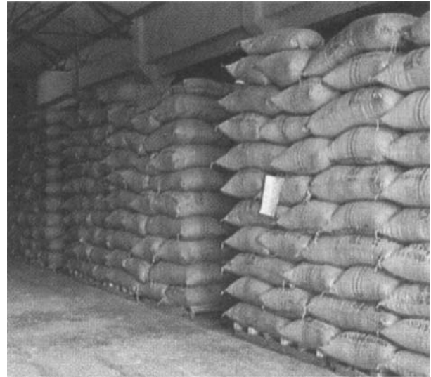
Fig.D.17: Platform of wooden planks used in godowns for storage of goods.
