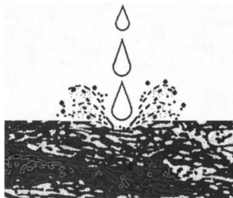
Fig.S.21: Raindrops cause splashing of soil particles and may lead to soil erosion.
