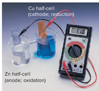
Figure 21.6 Measuring the standard cell potential of a zinc-copper cell.
