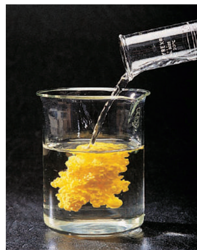
Figure 4.9 The precipitation of \text{PbI}_2 , a metathesis reaction.
