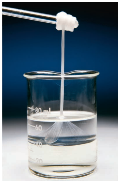
Figure 15.28 The formation of nylon-66. In the laboratory, the six-C diacid chloride, which is more reactive than the diacid, is used as one monomer; the polyamide forms between the two liquid phases.
