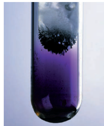
Figure 12.9 Iodine subliming. As the solid sublimates, I_2 vapor deposits on a cold surface (water-filled inner test tube).
