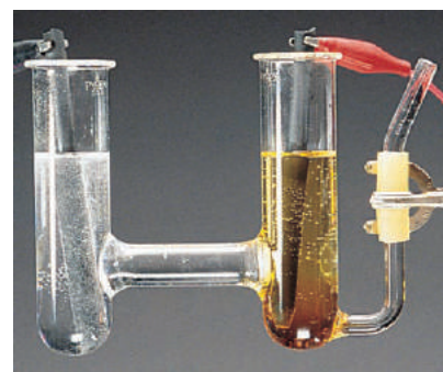
Electrolysis of aqueous KBr.
