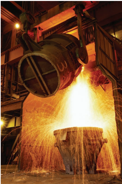
Figure 22.18 The basic-oxygen process for making steel.
