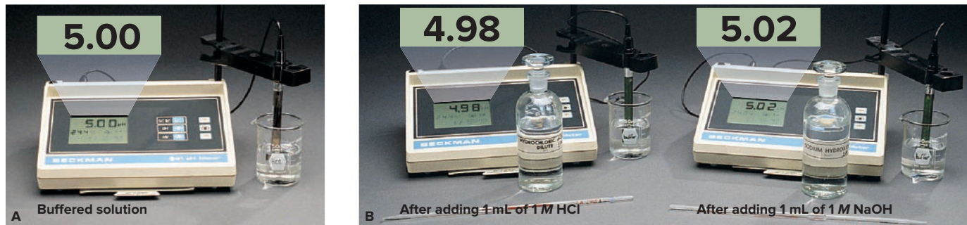
Figure 19.2 The effect of adding acid or base to a buffered solution. A , A 100-mL sample of an acetate buffer, which was made by mixing 1 M \text{CH}_3\text{COOH} with 1 M \text{CH}_3\text{COONa} , is adjusted to pH 5.00. B , Adding 1 mL of strong acid (left) or of strong base (right) changes the pH negligibly. Source: © McGraw-Hill Education/Stephen Frisch, photographer
