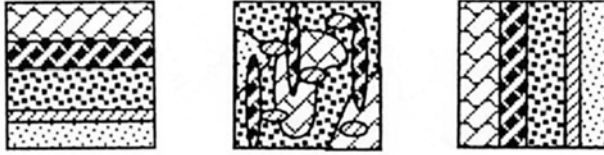
Fig. 14.13. Schematic representation of the series bound ( left ) and parallel bound ( right ) methods for a material comprising several phases. The medium is represented by a succession of layers each of which has a volume fraction corresponding to that of the phase it represents. The properties of the actual material necessarily lie between those of its two extreme representations
