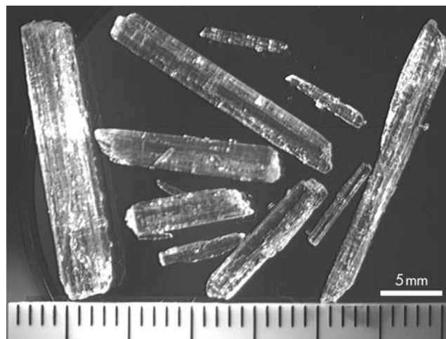
Figure 1: Photomicrograph of large dl -menthol crystals; magnification 7×. Manufacturer: Charkit Chemical Corp., USA.
