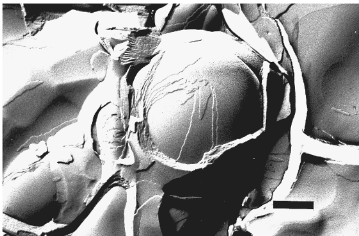
FIG. 13. Transmission electron micrograph of a freeze fractured w/o cream. The aqueous phase is dispersed as droplets within the continuous lipophilic phase; the interface consists of multiple bilayers of hydrated surfactant molecules, bar 500 nm. From Müller-Goymann, C., Halbfeste emulsionsähnliche Zustände, Seifen, Öle, Fette, Wachs , 110:395–400 (1984).
