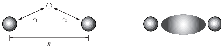
FIGURE 6.6 ▶ Left: general arrangement of three bodies, in this case two protons and an electron. Right: minimum energy configuration for \text{H}_2^+ . The electron is delocalized.
