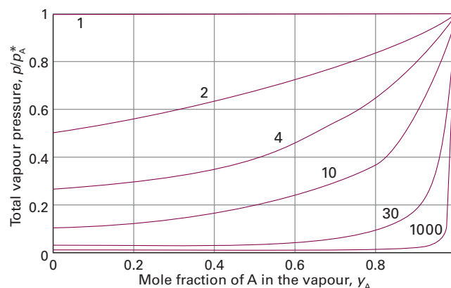
Figure 5C.3 The dependence of the vapour pressure of the same system as in Fig. 5C.2, but expressed in terms of the mole fraction of A in the vapour by using eqn 5C.5. Individual curves are labelled with the value of p_A^*/p_B^* .
