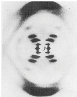
Fig. 19.42 The X-ray diffraction pattern obtained from a fibre of B-DNA. The black dots are the reflections, the points of maximum constructive interference, that are used to determine the structure of the molecule. (Adapted from an illustration that appears in J.P. Glusker and K.N. Trueblood, Crystal structure analysis: A primer . Oxford University Press (1972).)
