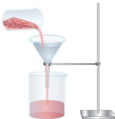
Figure 1: Separating solid from solution by filtration. (Source: CK-12 Foundation, License: CC-BY-SA)
