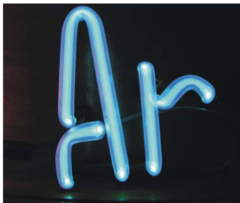
Figure 6: When an electric current is passed through argon gas, the gas glows blue. (Source: http://en.wikipedia.org/wiki/Image:Ar-Tube.jpg , License: CC-BY-SA) (
