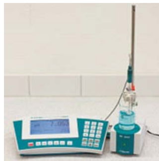
Figure 2B: An electronic pH meter (Source: http://commons.wikimedia.org/wiki/File:PH_meter.jpg , Author: Datamax, License: Public Domain)
