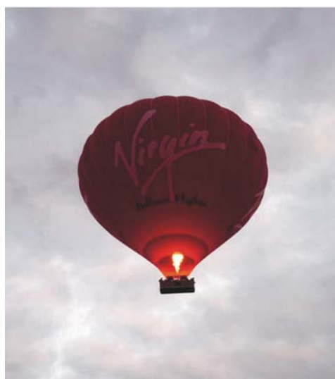
Figure 5: A hot air balloon transfers energy in the form of heat from the flame to the air particles in the balloon. The design of the hot air balloon takes this energy and changes it from heat to work. (Source: http://en.wikipedia.org/wiki/Image:Virgin_Hot_Air_Balloon.jpg , License: Public Domain)
