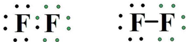
Figure 4: We can also show a covalent bond between atoms with an electron dot formula where the shared pair of electrons are the bonding electrons or with the bond represented by a dash.
