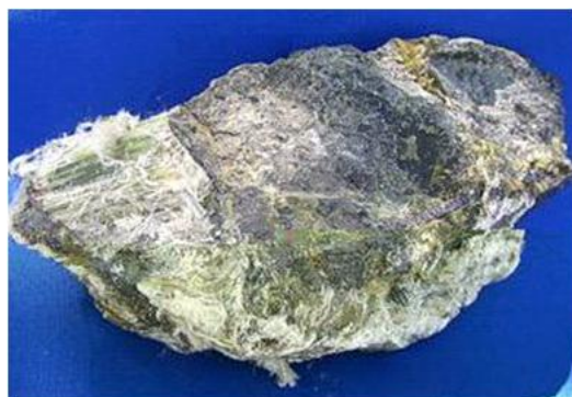
Figure 8: Asbestos in the form of chrysotile. You can see fibers of asbestos in the upper left hand corner of the photo.
