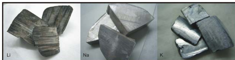
Figure 5: Notice how the elements lithium (Li), sodium (Na) and potassium (K) all look alike. They are all soft, silver metals. Since Li, Na and K are all Group 1A metals, they all share similar chemical properties.
