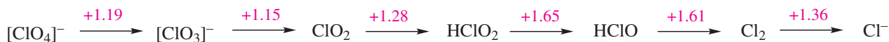
Fig. 7.7 Potential diagram (Latimer diagram) for chlorine in aqueous solution at pH 0, i.e. [\text{H}^+] = 1 \text{ mol dm}^{-3} .
