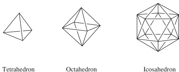
Fig. 3.8 The tetrahedron ( T_d symmetry), octahedron ( O_h symmetry) and icosahedron ( I_h symmetry) possess four, six and twelve vertices respectively, and four, eight and twenty equilateral-triangular faces respectively.
