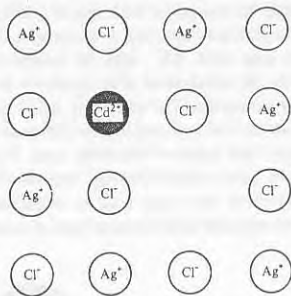
Fig. 7.11 Schottky defect (cation vacancy) induced and balanced by the presence of a higher valence cation. [Hannay, N. B. Solid-State Chemistry ; Prentice-Hall: Englewood Cliffs, NJ, 1967. Reproduced with permission.]
