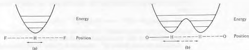
Fig. 15.51 Energy and position of the hydrogen atom in (a) the symmetric \text{HF}_2^- system and (b) an unsymmetric \text{O-H}\cdots\text{O} system. In (a) the average position of the hydrogen atom is midway between the fluoride ions. In (b) the positional sketch on the left represents the average position of the hydrogen in the left potential well and the dotted sketch represents the average position for the other potential well. The height of the energy barrier is qualitative and not meant to represent any particular system.
