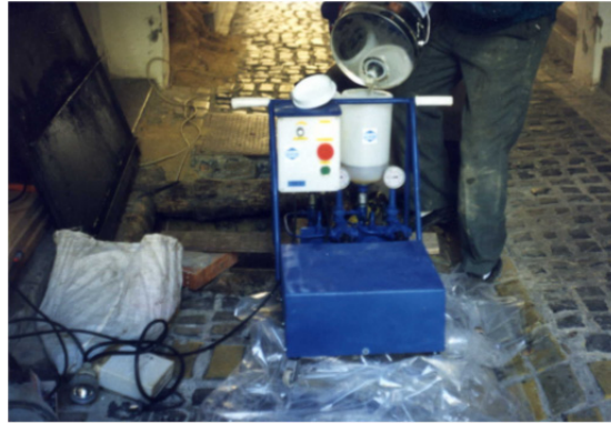
Figure 1. Two component electric grouting pump DV 97.
