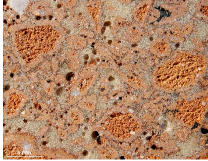
Figure 8. Diffusive porous zonal texture of geocomposite (crushed brick + PUR). A border formed by penetration of the binder into the pores of the brick fragments is visible on the bigger grain edges. Smaller brick fragments are fully penetrated by the binder.
