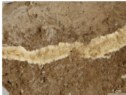
Figure 7. Claquage texture – fine-grained soil fractured hydraulically with claquage fissure, which is filled with PUR-binder.
