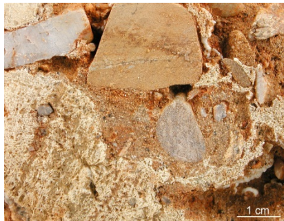
Figure 9. Barrier texture – the binder fills the interconnected cavities between the grains, it does not penetrate through the barriers formed by the basic mass.
