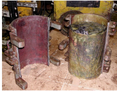
Figure 14. Sample of model geocomposite (PUR+basalt aggregate) prepared in laboratory by grouting into pressure tank.
