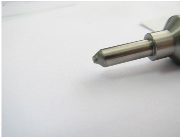
Figure 10. Mixing head needle corrosion by EG
