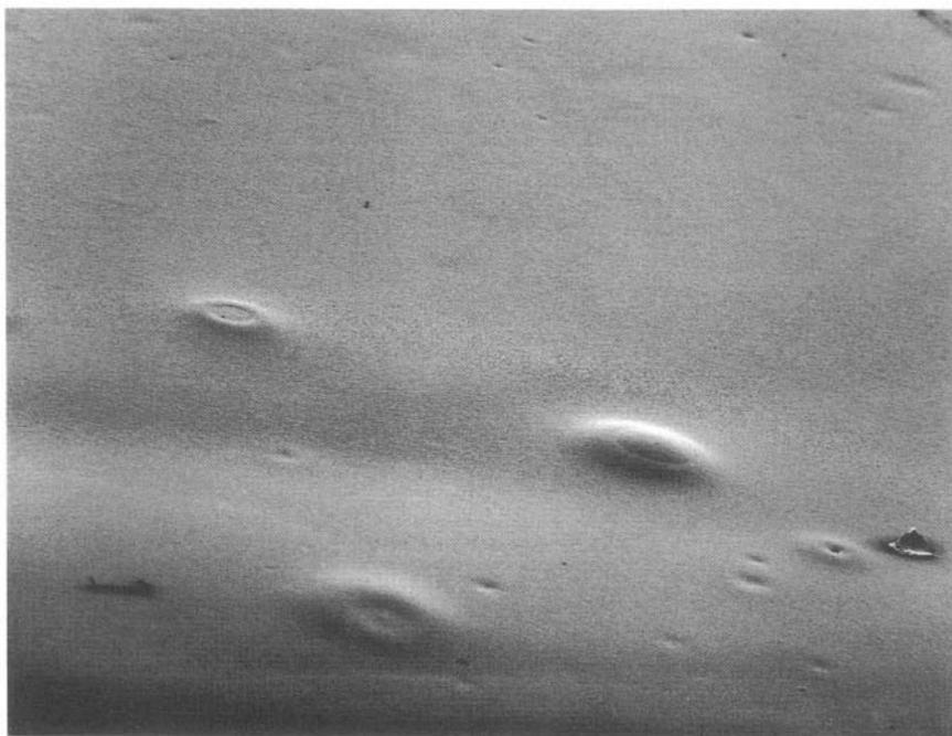
*Figure 3.3.* Scanning electron micrograph of air-oxidized alkyd IV emulsion, non-catalyzed, 50x magnification.
